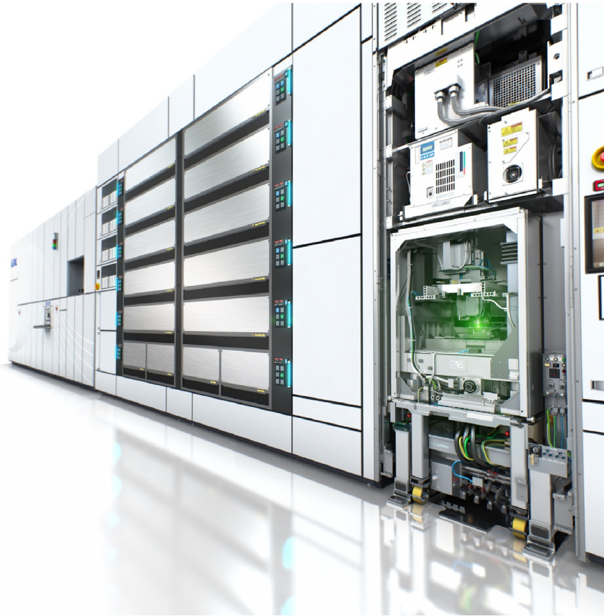
Fig. 23. YIELDSTAR Metrology system allows real-time chip property measurements enabling a closed-loop rejection of process disturbances.
